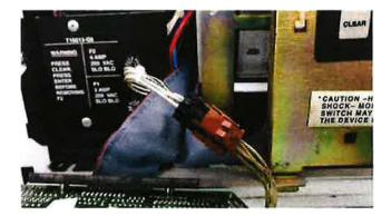
3. Disconnect the P801 Display Data cable from the SID Main Display.
