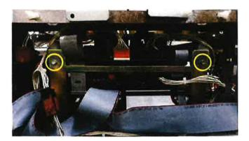
3. Disconnect the cables from the P201, P205 and P203 connectors on the SID Pump Controller board. Disconnect the Display Ribbon cable from the P204 connector and remove the cable from the Modular head to be discarded.
