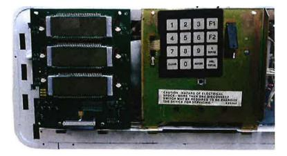
8. Before replacing the bezels, reapply power to the Modular head to ensure that the LCD Main Displays are working properly.
