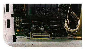
4. Remove the SID Main Display from the Modular head. Remove the mounting bracket from the bottom of the SID Main Display.
