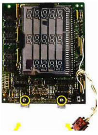
5. Install the bracket onto the M15224A001-8999 LCD Main Display and set aside for now.
