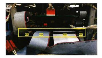
4. Remove the SID Pump Controller board by sliding the board away from the Modular Card cage.
