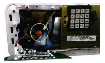
7. Mount the M15224A001-8999 LCD Main Display to the Modular head and reattach the Operator Panel Assembly to the unit.
