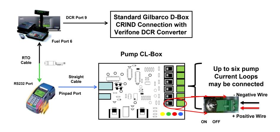
Note: All VX510 COM cables are pinned differently & CAN NOT be interchanged!!!
